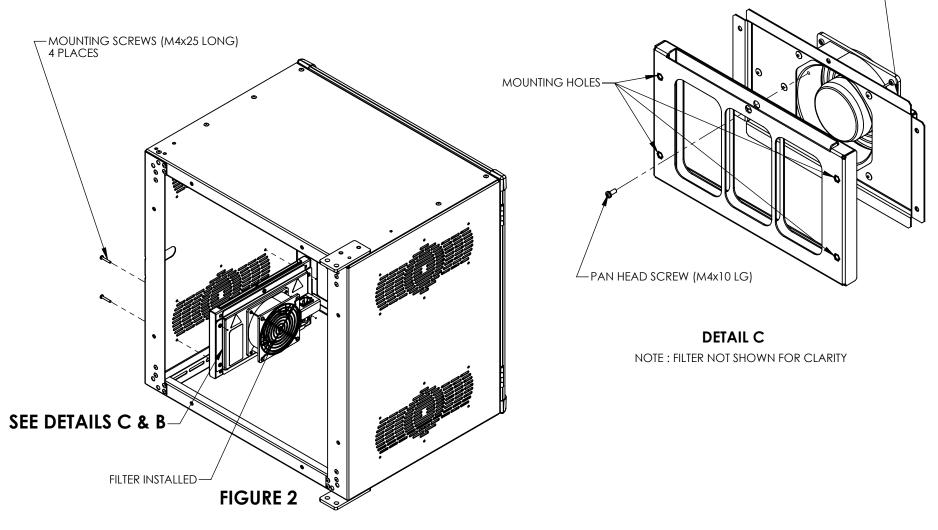
\*\* NOTE THAT WHEN MOUNTING BOTH (FILTER AND FAN KIT) ON THE INSIDE OF THE CABINET, THE BOTTOM THREE (3) RMU'S ARE RESTRICTED TO SHALLOW EQUIPMENT THAT DOES NOT BLOCK THE FAN EXHAUST.
